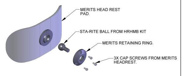
2. ASSEMBLE HEAD REST WITH STA-RITE BALL AS SHOWN. LOOSELY TIGHTEN 3 CAP SCREWS.
