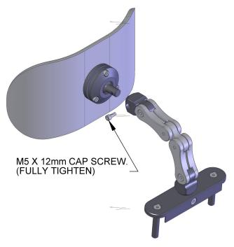
4. INSERT ASSEMBLY INTO CAPTAIN SEAT ALL THE WAY DOWN UNTIL UNTIL YOU HEAR EACH SIDE CLICK IN PLACE. ADJUST HEAD PAD ANGLE (3 SCREWS) AND ARM ANGLES (4 SCREWS), AS REQUIRED. FULLY TIGHTEN ALL SCREWS AFTER ADJUSTMETS ARE COMPLETE.
